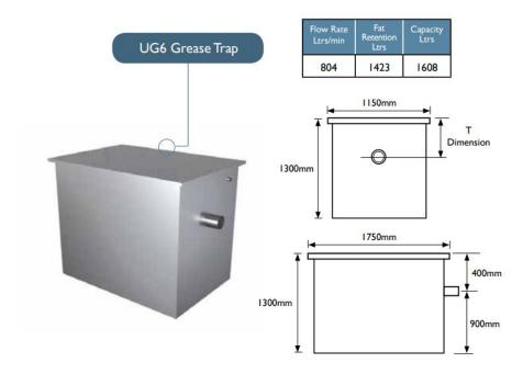
When used under floor cover is set to suit floor finish inlet/outlet to suit drainage under slab, a support arrangement can be fitted using threaded bar & M/S angle.
