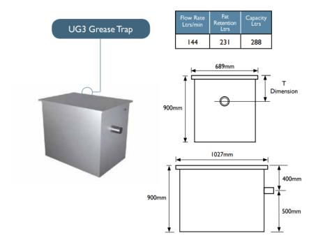
When used under floor cover is set to suit floor finish inlet/outlet to suit drainage under slab, a support arrangement can be fitted using threaded bar & M/S angle.
